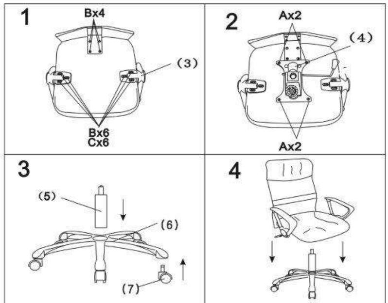
It is important to assemble all parts so that the directional "Arrows" point in the same direction. Make certain that all screws are FULLY tightened before using the chair. Each month check all screws and tighten and that may have loosened.
